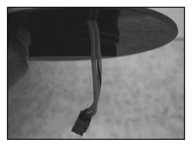
2) Plug in-line Euro-block connector(s) to chassis-mount input connector(s) on speaker.
