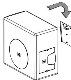
6. Remove the input terminal cover, connect wiring and set the tap selector rotary switch. Replace input terminal cover, routing wires through the side opening, dressing the wiring toward the back side of the cabinet.
