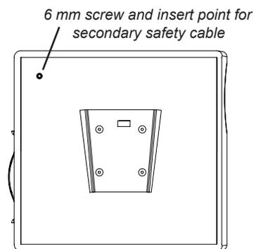
5. Position Control 50S/T subwoofer toward wall, in the orientation shown, slightly higher than the on-wall plate, then slide the Control 50S/T subwoofer downward while maintaining pressure toward the wall until the two bracket plates engage. Make sure the retaining spring latches securely into place.
